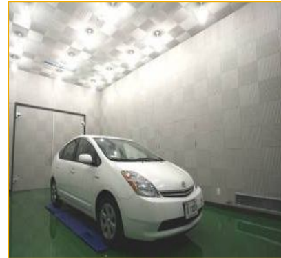
Vehicle Noise Test Room
