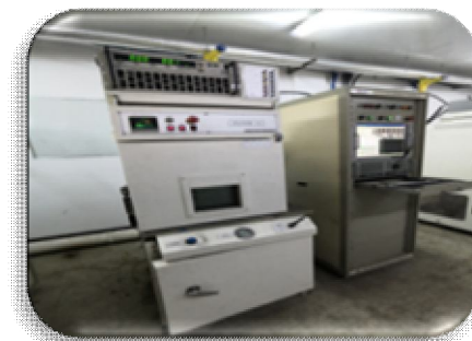
Alternator Durability tester
