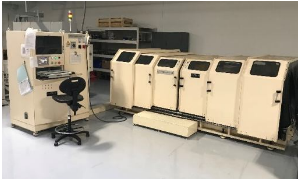
Torsional fatigue tester
