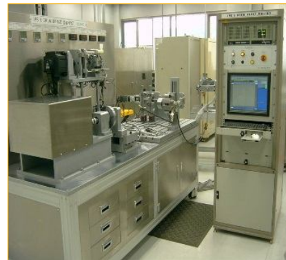
Caliper Brake Performance
